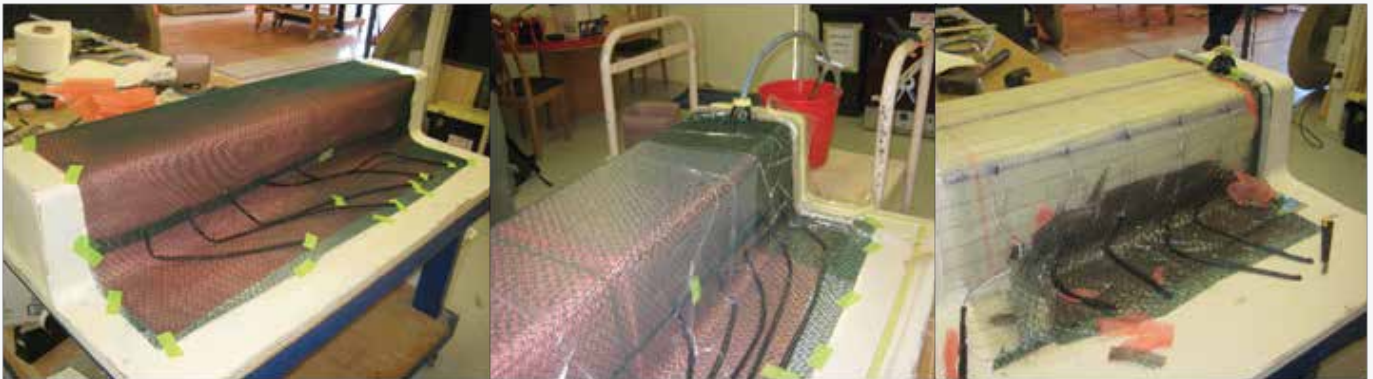
Figure 9: (a) Preparation for VIP; (b) Infusion process; (c) Specimen with embedded FBGs, bag removal process
