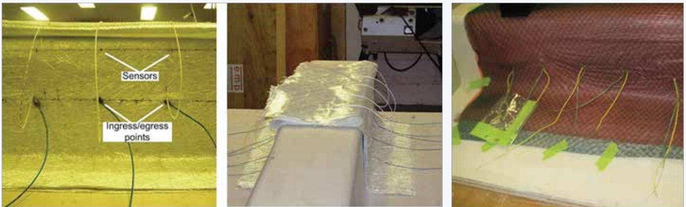
Figure 8: (a & b) Positioning of bare FBG sensors on the marked area; (c) specimen ready for infusion
