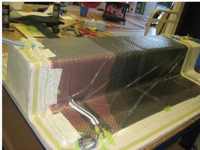
Figure 3: Top-hat-stiffener manufacturing with VARTM
